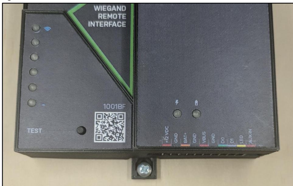
Figure 15: Bottom DIN Rail Screw Mount
