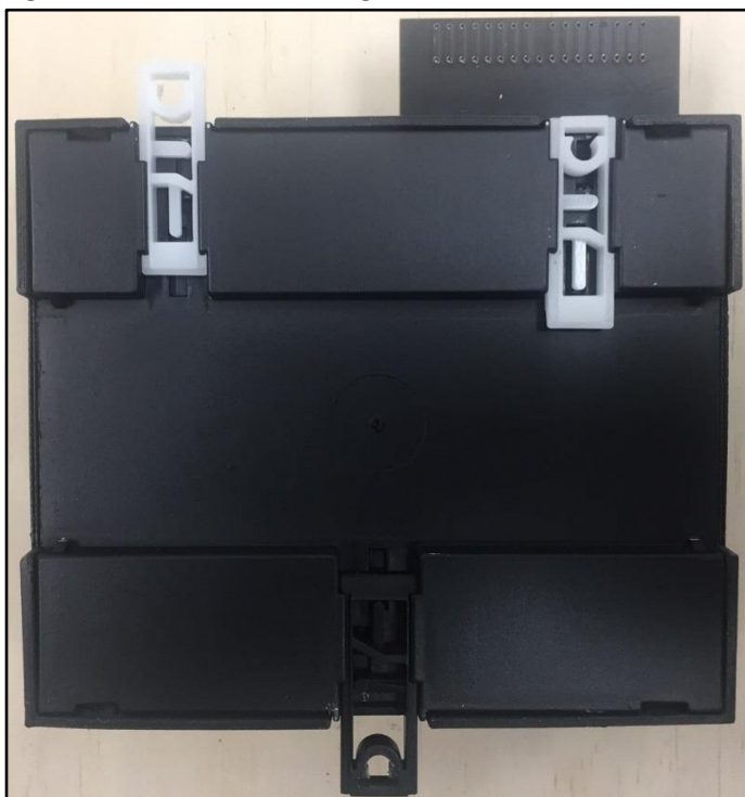
Figure 13: DIN Rail Mounting Pins
